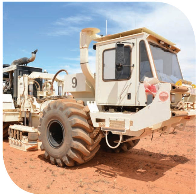
Image: Terrex Seismic's INOVA AVH IV Vibrator at ATP 594 Harrier 3D Seismic Survey.
